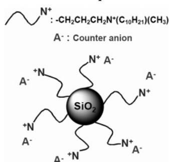
Chart 1. Schematic Structure of Silica Nanoparticle Based Ionic Liquid
